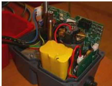
Following a battery driven cycle the actuator will need to charge for a short period to replace the energy used in the battery cycle.
