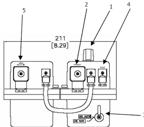
**On/off, fails safe on power failure:**
