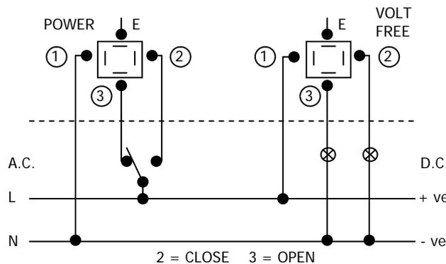
**Wiring Diagram (AC or DC): 3 wire**
