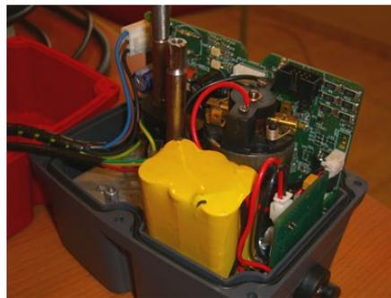
Following a battery driven cycle the actuator will need to charge for a short period to replace the energy used in the battery cycle. This is particularly relevant if you intend to use the **J3** -BSR like a solenoid, eg: energise open, fail close.
