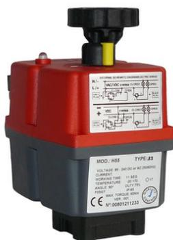
Protection against valve jams is provided by an electronic torque limiter, which auto-relaxes the gearbox when activated, allowing the manual override to be selected
