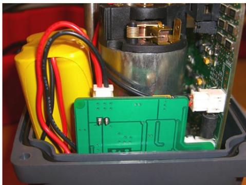
at full strength from an internal trickle charging system.
