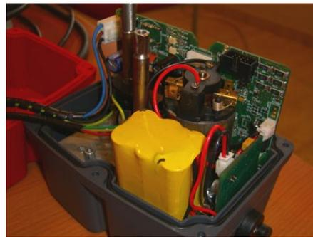
Following a battery driven cycle the actuator will need to charge for a short period to replace the energy used in the battery cycle. This is particularly relevant if you intend to use the **J3** -BSR like a solenoid, eg: energise open, fail close.
