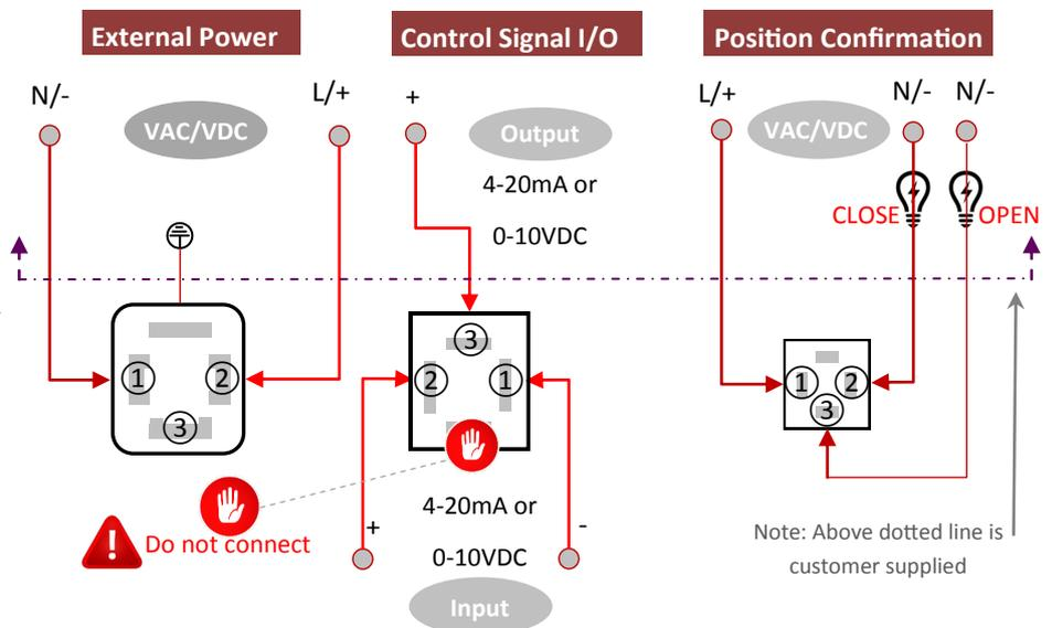
**J3C FAILSAFE MODULATING ACTUATOR**
