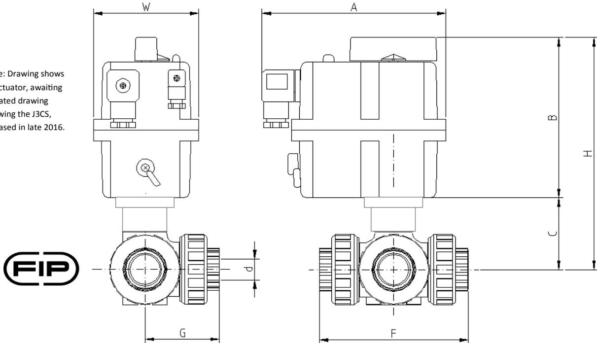
Type: **E3416FS** Actuator fitted to valve via the 'EasyFit-F' mounting kit manufactured by J+J
