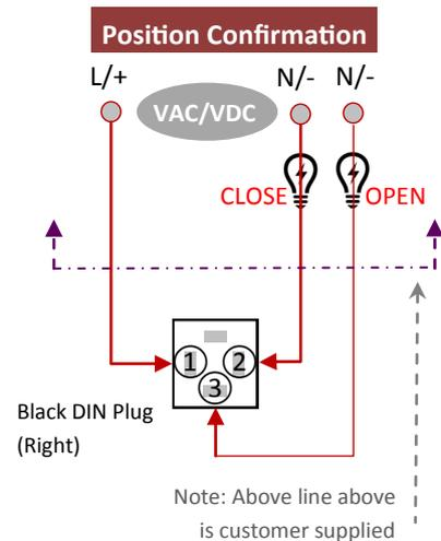
In J+J electric actuators all electrical connections are made externally using the external DIN plugs supplied with the actuator. There is no need to remove the valve actuator's cover to connect electrically. There are no terminals internally to connect to.
