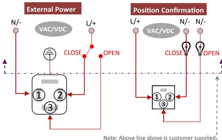
In J+J electric actuators all electrical connections are made externally using the external DIN plugs supplied with the actuator. There is no need to remove the valve actuator's cover to connect electrically. There are no terminals internally to connect to.
